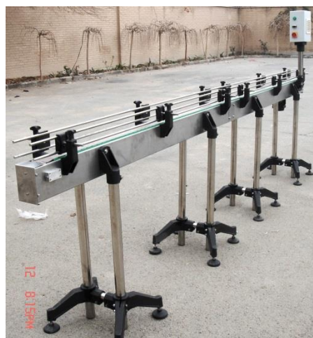
Wide width Conveyor with modular chain
